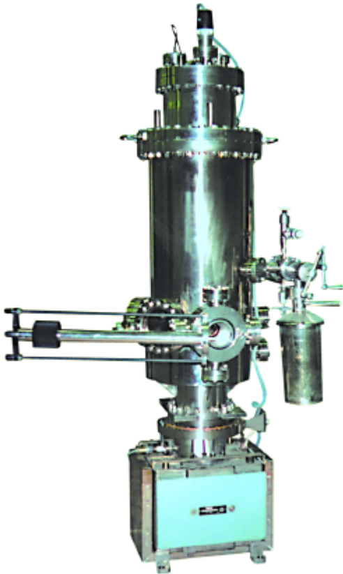
Low-temperature UHV SPM inside ultra high vacuum helium cryo-pump
