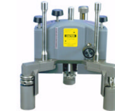
The head for scanning by the cantilever
