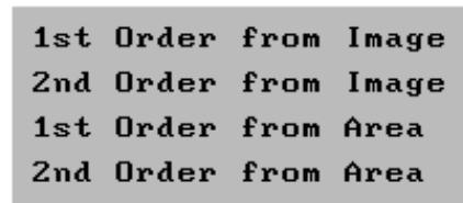
“1st Order from Image” fitted plane subtraction. This operation eliminates the inclination effect appearing as a result of nonparallelism of the scanning plane and surface plane.
