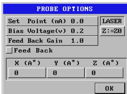
“**SetPoint (nA)**” sets the current value to be maintained constant by feedback (tunnelling current for the STM mode and photodiode differential current for the SFM mode).
